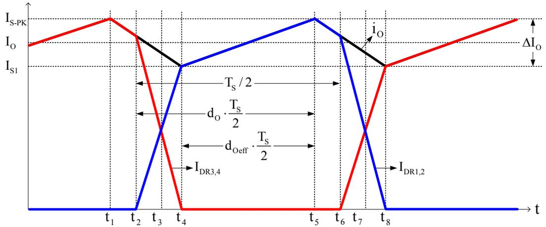
Figure 4.6 The rectifier diode and load current waveforms.
