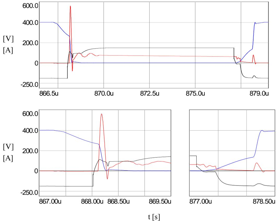
Figure 5.19 Lagging leg IGBT module ( $T_2$ ) waveforms at 15% load (top, same as Figure 5.18), and the detailed turn-on and turn-off switching transitions of this module (bottom).
