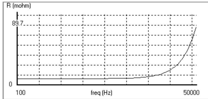
Figure 4.9 The primay winding resistance obtained by FEA.
