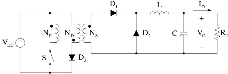
Figure 2.7 The forward DC/DC converter circuit configuration.
