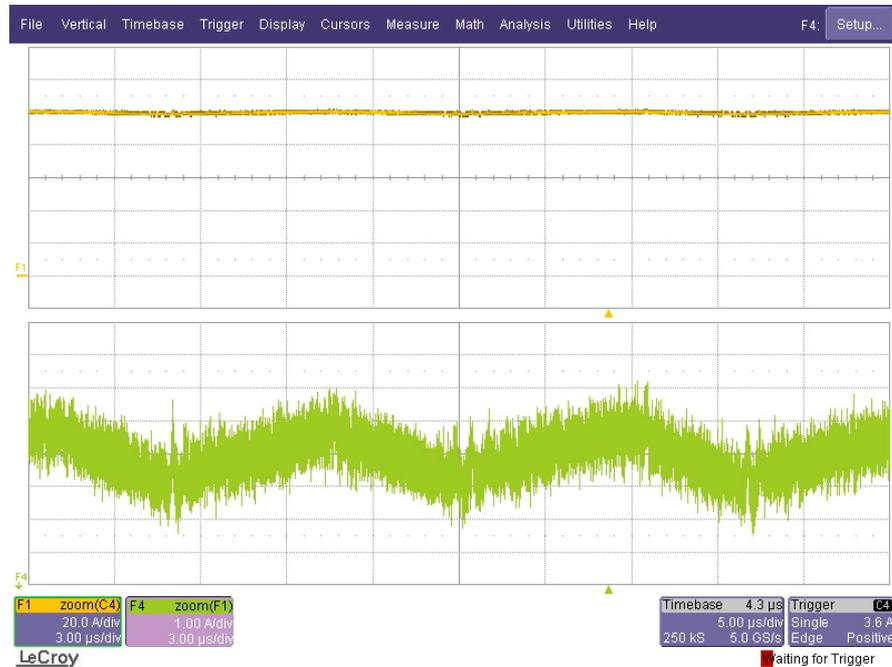
Figure 6.8 Load current waveform (top) and its vertically zoomed version (bottom) at the rated load current (scales: 20 A/div, 1 A/div, 3  $\mu$ s/div).
