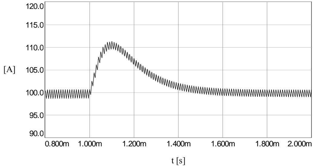
Figure 5.29 Load regulation performance of the output current controller.
