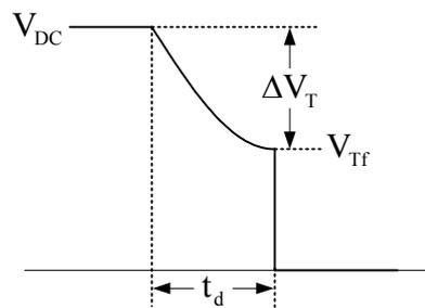
Figure 4.4 The switch voltage waveform during hard-switching.
