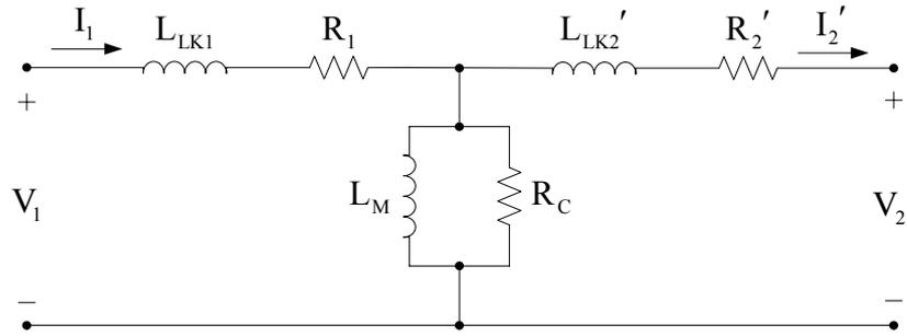
Figure 4.12 Primary referred transformer T equivalent circuit.
