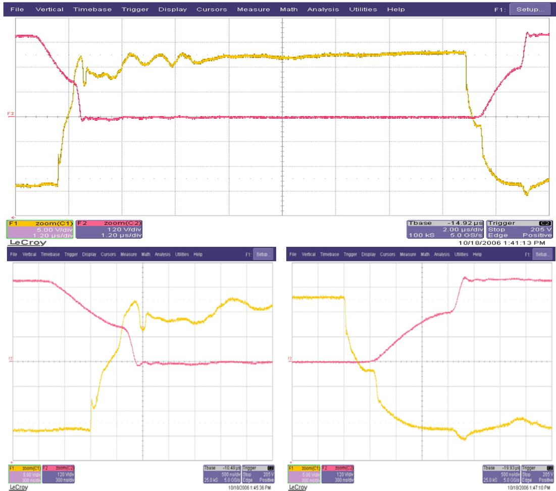
Figure 6.22 Collector-emitter voltage (red) and gate-emitter voltage (yellow) waveforms of the lagging leg IGBT ( $T_2$ ) (top; scales: 120 V/div, 5 V/div, 1.2  $\mu$ s/div), and the turn-on and turn-off switching transitions of this IGBT (bottom; scales: 120 V/div, 5 V/div, 300 ns/div) at 25% load.
