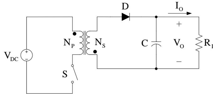
Figure 2.6 The flyback DC/DC converter circuit configuration.
