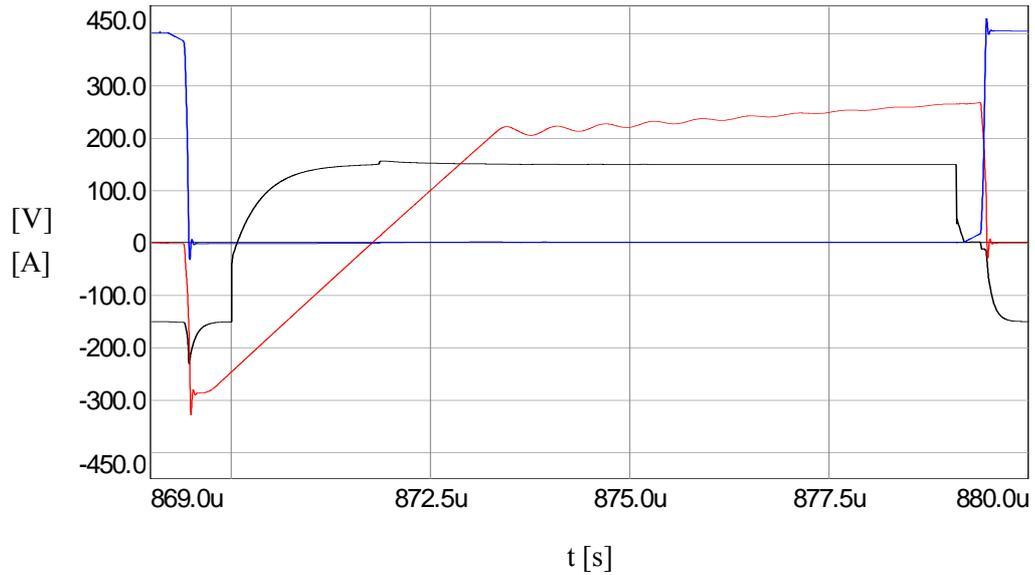
Figure 5.6 Leading leg IGBT module ( $T_4$ ) waveforms at the rated load current:
