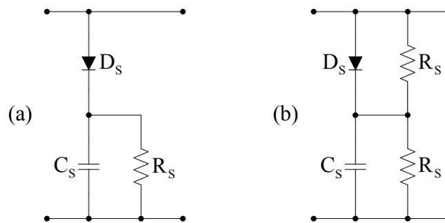
Figure 6.30 Voltage clamp snubbers utilized for performance comparison.
