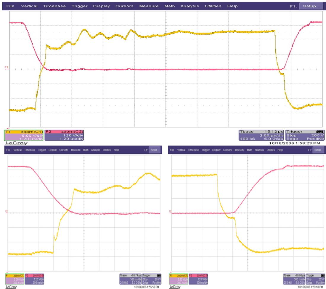
Figure 6.16 Collector-emitter voltage (red) and gate-emitter voltage (yellow) waveforms of the lagging leg IGBT ( $T_2$ ) (top; scales: 120 V/div, 5 V/div, 1.2  $\mu$ s/div), and the turn-on and turn-off switching transitions of this IGBT (bottom; scales: 120 V/div, 5 V/div, 300 ns/div) at the critical load current.
