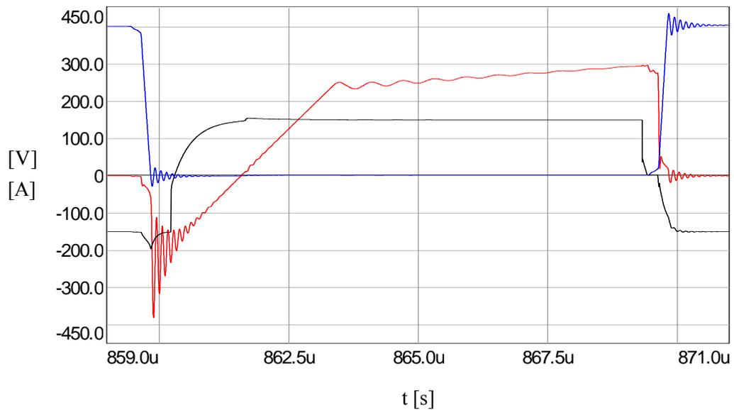
Figure 5.7 Lagging leg IGBT module ( $T_2$ ) waveforms at the rated load current:
