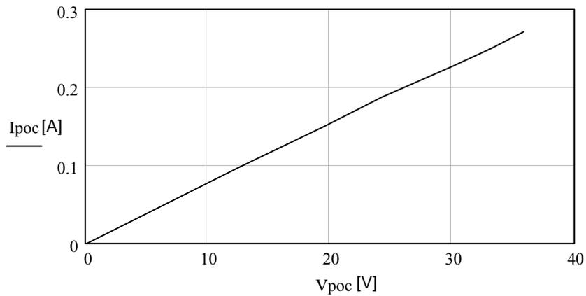
Figure 4.16 The primary current ( $I_{poc}$ ) versus the primary voltage ( $V_{poc}$ ) obtained from the open-circuit test.
