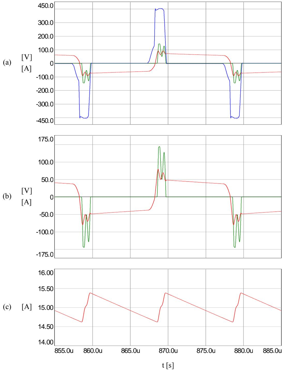
Figure 5.16 FB-PS-ZVS DC/DC power converter waveforms at 15% load:
