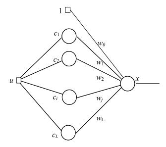
Figure 9.4 Single input, single output RBF network
