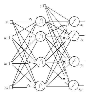
Fig. 9.1. Structure of the Standart RBF network
