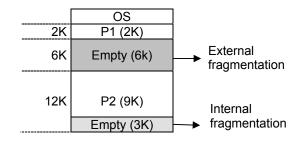
In this composition of memory, if a new process, P3, requiring 8 KB of memory comes, although there is enough total space in memory, it can not be loaded because fragmentation.
