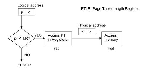
Given a logical address to access the word in physical memory, first access the PT stored in registers, which requires register access time (rat), and then find out the physical address and access the physical memory, which requires memory access time (mat). Therefore effective memory access time (emat) becomes:
