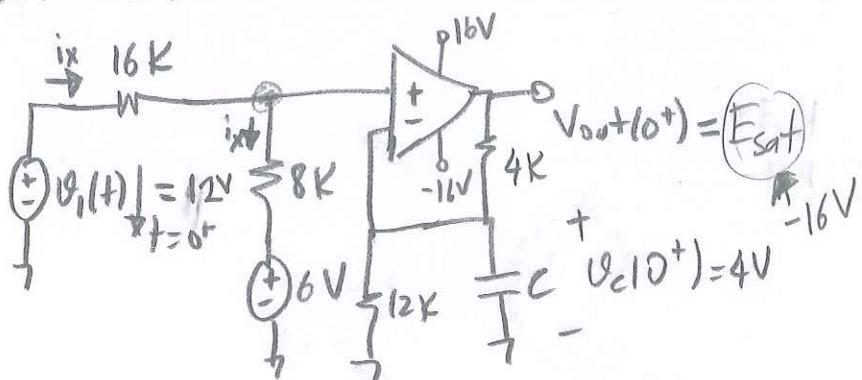
$$\vartheta_+ = ? \quad i_x = \frac{12-6}{24} \text{ mA} = \frac{1}{4} \text{ mA}$$
