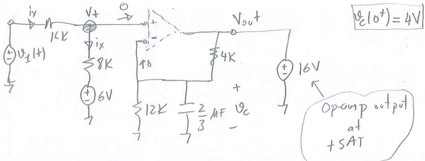
$$(1) V_+ = 6 + \left( \frac{V_1 - 6}{24} \right) 8 = \frac{V_1}{3} + 4 \text{ Volts,}$$
