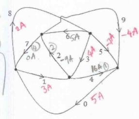
The figure on the left shows the oriented graph of a lumped circuit.
