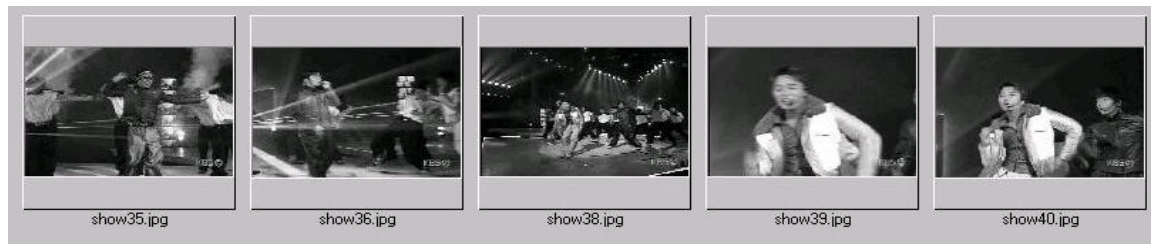
Figure 6. 5 shots out of 600 that have highest (act_1 - act_0) difference. Note that, act_0 , also act_1 to some degree, is misled by camera motion. We are able to filter out high camera motion segments by using the (act_1 - act_0) difference.
